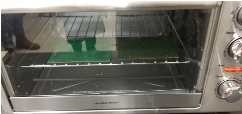
Figure 21A. PCB inside oven after coating.
