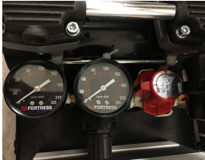
Figure 27A. Close up picture of air gauge that should reach 20 psi.
