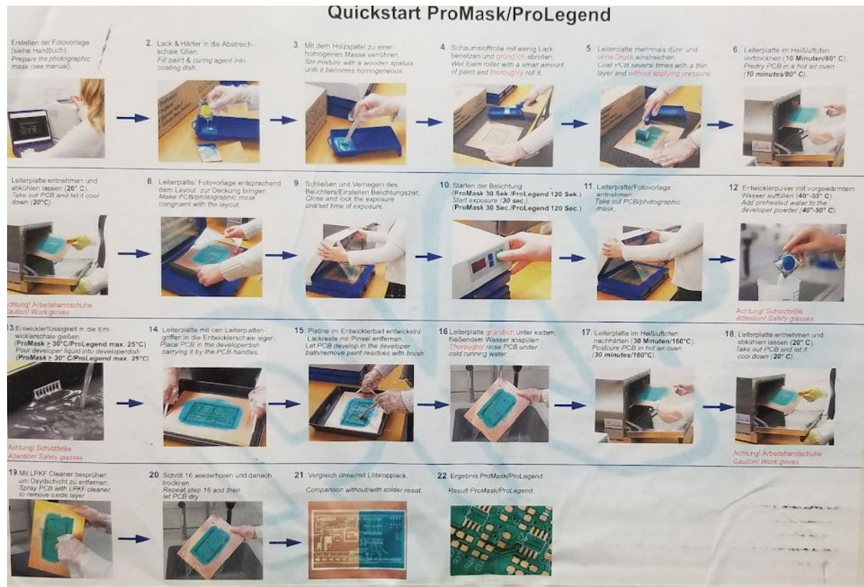
Figure 22A. Masking procedure at the UTA laboratory.
